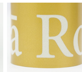
Skirt off-set printed decoration on metallic side base-coat.
